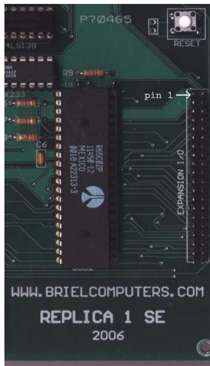
replica 1 showing pin 1 location
