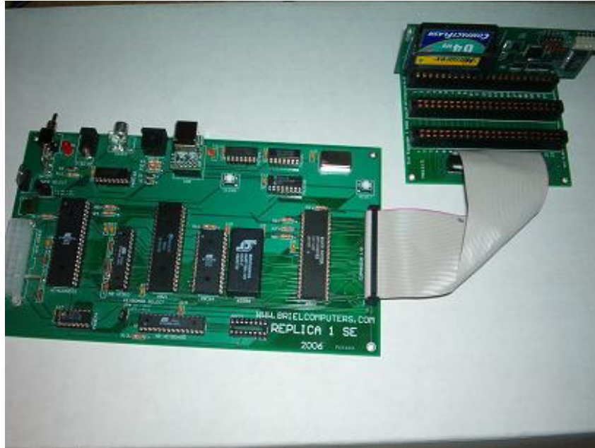
replica 1 shown with correct cable orientation
